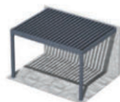
Wall-mounted blades perpendicular to wall
