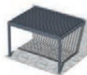
Wall-mounted blades perpendicular to wall
